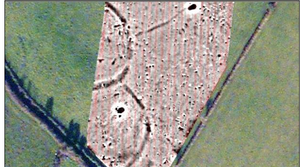
5. GPS tracks (red) highlighting lines of data collection & results from magnetometer fieldwork at a suspected burial ground.
